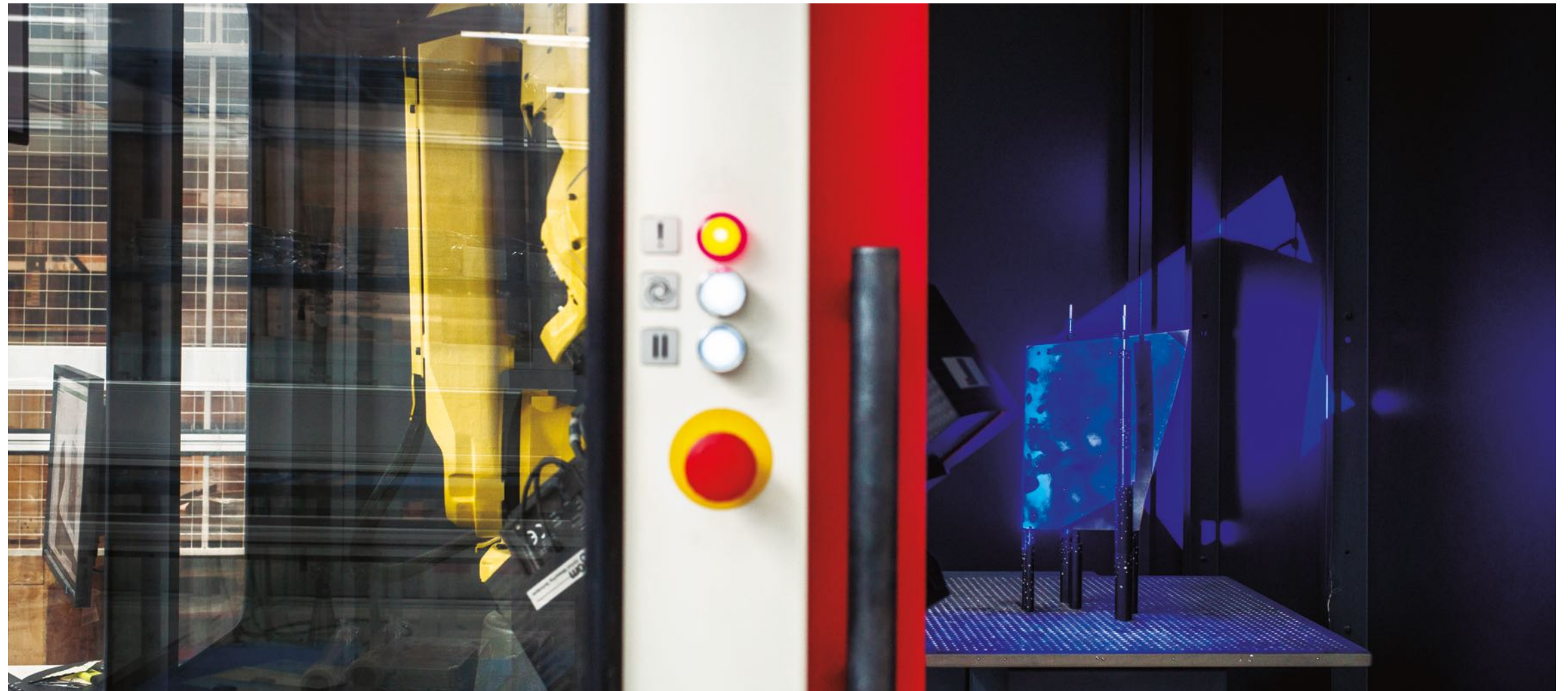
Dimensional Measuring Machine (non-contact) GOM.
