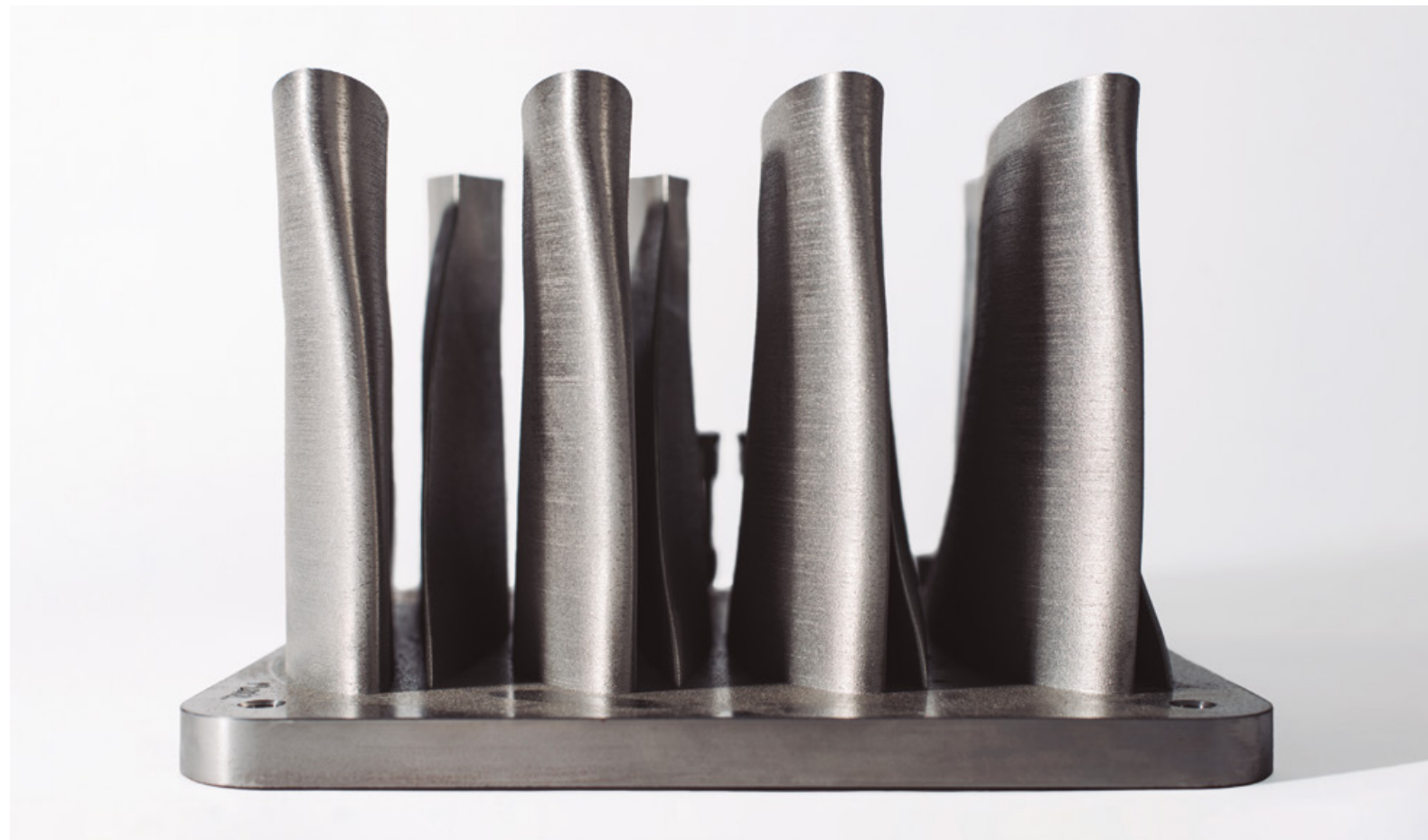
Components designed and manufactured using additive technology.
