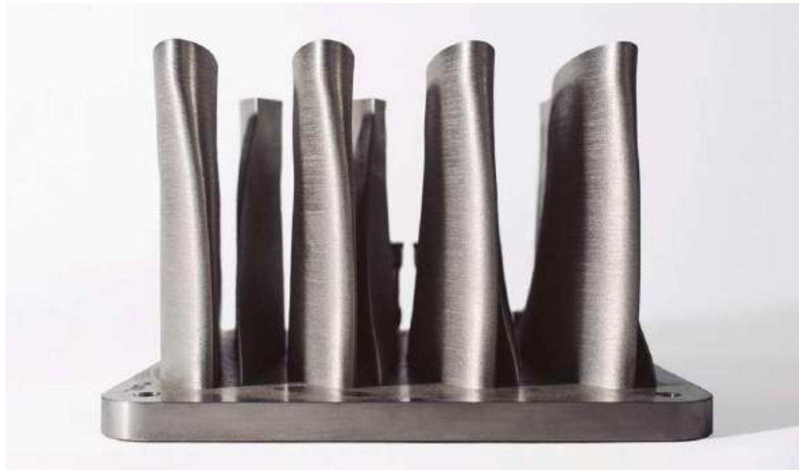
Components designed and manufactured using additive technology.
